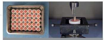
**Figure 1.** Shear bond testing of porcelain and composite discs embedded in polymethyl methacrylate blocks
